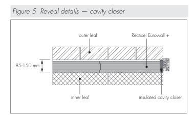
14.14 Additional wall ties at 300 mm vertical centres within 225 mm of all openings are recommended in BS EN 1996-1-1 : 2005 and BS EN 1996-1-2 : 2005. For this product, this would involve piercing the boards and may introduce an unacceptable risk of water penetration. Therefore, it is recommended that an additional wall tie is included within 225 mm of the opening on each board course level to satisfy the structural requirements of the wall (see Figure 6).
