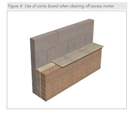
14.11 The boards can be cut, using a sharp knife or fine-toothed saw, to fit openings, eg around windows, doors and airbricks. It is essential that cut pieces completely fill the spaces for which they are intended and are adequately secured.
