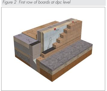
Figure 2 First row of boards at dpc level
