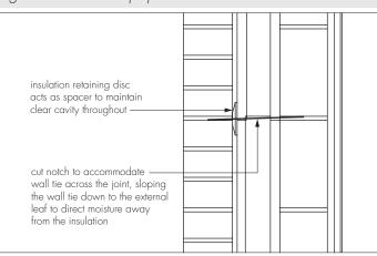
14.4 The boards incorporate a tongue-and-groove edging so that each subsequent row of boards interlocks tightly with the previous row by slotting the tongue-and-groove edges together in a jigsaw effect. The two distinct facers, one a grey alkali-resistant coating placed against the inner leaf, the other a low emissivity multi-layer aluminium facing the cavity airspace, help the installer to fit the boards the right way up with the horizontal tongue joint facing upwards (see Figure 3).
